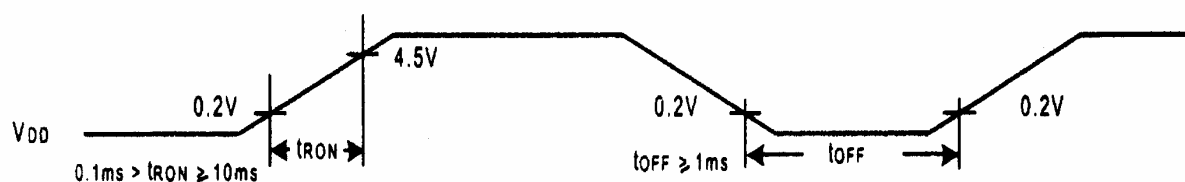
Figure 4. t_{OFF} stipulates the time of power OFF for instantaneous power supply to or when power supply repeats ON and OFF.
