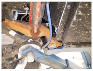
**Rear lifting point when replacing the battery:** On the damper fastening on the control arm ensuring enough space for the battery tray when the tray is lowered. The same on the opposite side.
