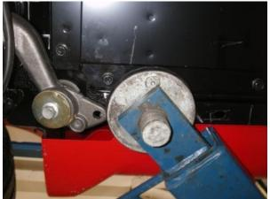
Rear lifting point when replacing the rear suspension
