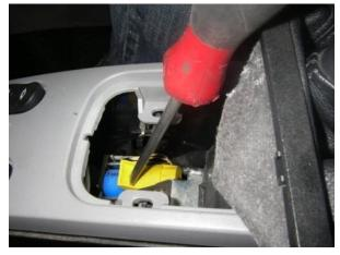
In an emergency the gearshift can be operated like this:
